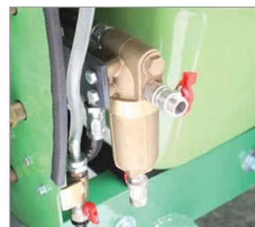
Pressure filter, with self-cleaning.
